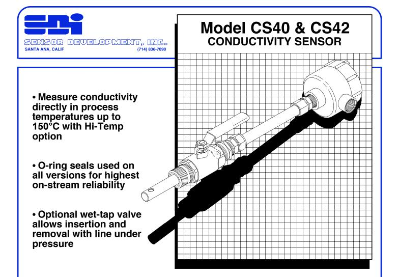
The Model CS40 & CS42 sensors have been designed for a wide measurement range in difficult process conditions. It can be installed in submersion, insertion, or wet-tap configurations, and is good for most applications from high purity water to high chemical concentrations.
